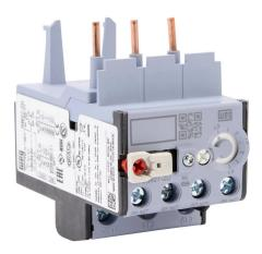
WEG Electric RW27-2D series thermal overload relay, 1.2-1.8A adjustable, bi-metallic, direct mount power connection(s). For use with CWB9 to CWB38 series contactors.
