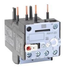
WEG Electric RW17-2D series thermal overload relay, 22.0-32.0A adjustable, bi-metallic, direct mount power connection(s). For use with CWC025 series miniature contactors.
