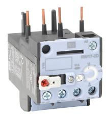
WEG Electric RW17-2D series thermal overload relay, 15.0-23.0A adjustable, bi-metallic, direct mount power connection(s). For use with CWC025 series miniature contactors.
