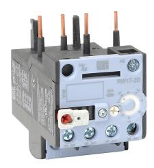
WEG Electric RW17-2D series thermal overload relay, 10.0-15.0A adjustable, bi-metallic, direct mount power connection(s). For use with CWC025 series miniature contactors.
