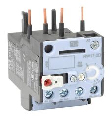
WEG Electric RW17-2D series thermal overload relay, 8.0-12.5A Adjustable, bi-metallic, direct mount power connection(s). For use with CWC025 series miniature contactors.
