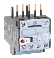
WEG Electric RW17-1D series thermal overload relay, 10.0-15.0A adjustable, bi-metallic, direct mount power connection(s). For use with CWC07 through CWC016 series miniature contactors.
