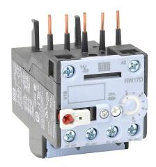
WEG Electric RW17-1D series thermal overload relay, 7.0-10.0A Adjustable, bi-metallic, direct mount power connection(s). For use with CWC07 through CWC016 series miniature contactors.
