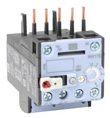
WEG Electric RW17-1D series thermal overload relay, 5.6-8.0A Adjustable, bi-metallic, direct mount power connection(s). For use with CWC07 through CWC016 series miniature contactors.
