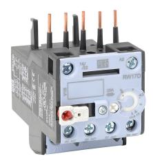
WEG Electric RW17-1D series thermal overload relay, 8.0-12.0A adjustable, bi-metallic, direct mount power connection(s). For use with CWC07 through CWC016 series miniature contactors.
