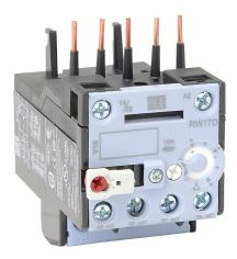
WEG Electric RW17-1D series thermal overload relay, 4.0-6.3A Adjustable, bi-metallic, direct mount power connection(s). For use with CWC07 through CWC016 series miniature contactors.
