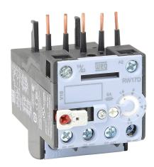
WEG Electric RW17-1D series thermal overload relay, 1.8-2.8A adjustable, bi-metallic, direct mount power connection(s). For use with CWC07 through CWC016 series miniature contactors.
