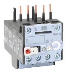
WEG Electric RW17-1D series thermal overload relay, 1.2-1.8A adjustable, bi-metallic, direct mount power connection(s). For use with CWC07 through CWC016 series miniature contactors.
