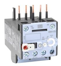
WEG Electric RW17-1D series thermal overload relay, 0.56-0.8A adjustable, bi-metallic, direct mount power connection(s). For use with CWC07 through CWC016 series miniature contactors.
