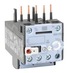
WEG Electric RW17-1D series thermal overload relay, 0.28-0.4A adjustable, bi-metallic, direct mount power connection(s). For use with CWC07 through CWC016 series miniature contactors.
