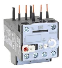
WEG Electric RW17-1D series thermal overload relay, 0.4-0.63A adjustable, bi-metallic, direct mount power connection(s). For use with CWC07 through CWC016 series miniature contactors.
