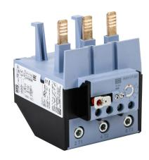
WEG Electric RW117-3D series thermal overload relay, 110.0-140.0A adjustable, bi-metallic, direct mount power connection(s). For use with CWB95 to CWB125 series contactors.
