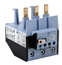
WEG Electric RW117-3D series thermal overload relay, 90.0-112.0A adjustable, bi-metallic, direct mount power connection(s). For use with CWB95 to CWB125 series contactors.
