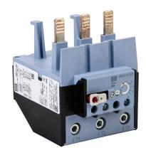
WEG Electric RW117-3D series thermal overload relay, 63.0-80.0A adjustable, bi-metallic, direct mount power connection(s). For use with CWB95 to CWB125 series contactors.
