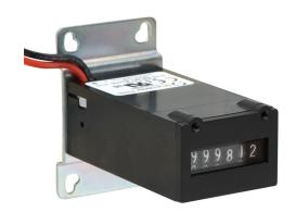
Trumeter electromechanical counter, 4mm 6-digit analog, 24 VDC input, rectangular 2-hole/4-hole base mount, (2) 11in 22 AWG pigtails.
