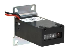
Trumeter electromechanical counter, 4mm 6-digit analog, 24 VDC input, rectangular 2-hole/4-hole base mount, (2) 11in 22 AWG pigtails.
