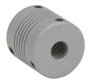
Koyo encoder coupling, 6mm bore, aluminum alloy body, setscrew. For use with Koyo TRD-S series encoders.
