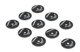
Contrinex basic RFID tag, round, 30mm diameter, non-flush mount, HF communication, 13.56 MHz, EEPROM memory, 320 bytes, IP68 IP69K. Package of 10.
