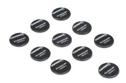
Contrinex basic RFID tag, round, 20mm diameter, non-flush mount, HF communication, 13.56 MHz, EEPROM memory, 320 bytes, IP68 IP69K. Package of 10.
