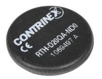
Contrinex basic RFID tag, round, 20mm diameter, non-flush mount, HF communication, 13.56 MHz, FRAM memory, 2048 bytes, IP68 IP69K.
