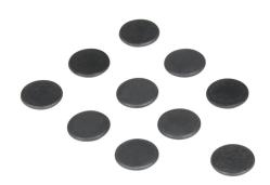
Contrinex basic RFID tag, round, 16mm diameter, non-flush mount, HF communication, 13.56 MHz, EEPROM memory, 320 bytes, IP67. Package of 10.
