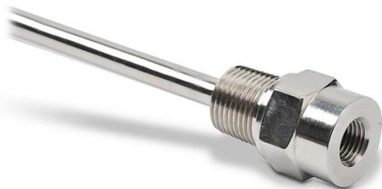
ProSense thermowell, 1/4in female NPT probe connection, 1/2in male NPT process connection, 316 stainless steel body, 213mm overall length, 7mm bore.
