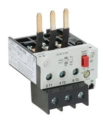
AutomationDirect RTD65 series thermal overload relay, 52.0-65.0A adjustable, bi-metallic, direct mount power connection(s). For use with GH15JT 60mm contactors.
