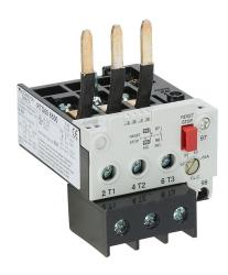
AutomationDirect RTD65 series thermal overload relay, 52.0-65.0A adjustable, bi-metallic, direct mount power connection(s). For use with GH15JT 60mm contactors.
