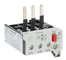
AutomationDirect RTD65 series thermal overload relay, 28.0-42.0A adjustable, bi-metallic, direct mount power connection(s). For use with GH15GT or GH15HT 60mm contactors.
