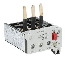
AutomationDirect RTD65 series thermal overload relay, 20.0-28.0A adjustable, bi-metallic, direct mount power connection(s). For use with GH15GT, GH15HT, or GH15JT 60mm contactors.
