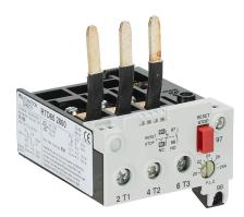
AutomationDirect RTD65 series thermal overload relay, 20.0-28.0A adjustable, bi-metallic, direct mount power connection(s). For use with GH15GT, GH15HT, or GH15JT 60mm contactors.
