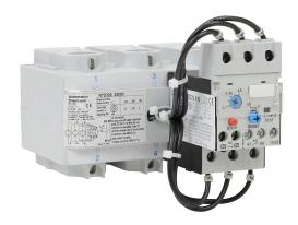
AutomationDirect RTD320 series thermal overload relay, 216.0-320.0A adjustable, bi-metallic, pass through connection(s), panel mount. For use with GH15ST or GH15TT 145mm contactors.
