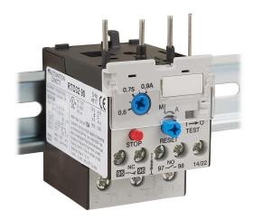
AutomationDirect RTD32 series thermal overload relay, 0.6-0.9A adjustable, bi-metallic, direct mount power connection(s), DIN rail mount. For use with GH15BN to GH15FT 45mm contactors.
