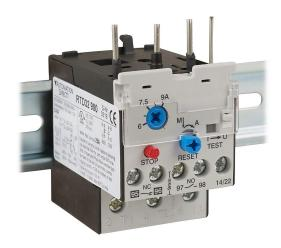
AutomationDirect RTD32 series thermal overload relay, 6.0-9.0A adjustable, bi-metallic, direct mount power connection(s), DIN rail mount. For use with GH15BN to GH15FT 45mm contactors.
