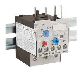
AutomationDirect RTD32 series thermal overload relay, 0.4-0.6A adjustable, bi-metallic, direct mount power connection(s), DIN rail mount. For use with GH15BN to GH15FT 45mm contactors.
