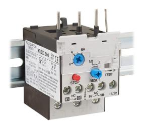
AutomationDirect RTD32 series thermal overload relay, 4.0-6.0A adjustable, bi-metallic, direct mount power connection(s), DIN rail mount. For use with GH15BN to GH15FT 45mm contactors.
