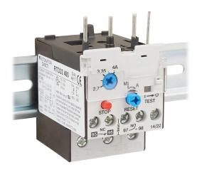
AutomationDirect RTD32 series thermal overload relay, 2.7-4.0A adjustable, bi-metallic, direct mount power connection(s), DIN rail mount. For use with GH15BN to GH15FT 45mm contactors.
