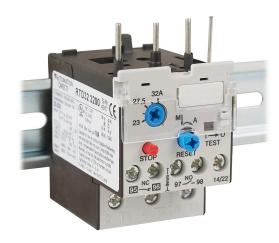
AutomationDirect RTD32 series thermal overload relay, 23.0-32.0A adjustable, bi-metallic, direct mount power connection(s), DIN rail mount. For use with GH15ET or GH15FT 45mm contactors.
