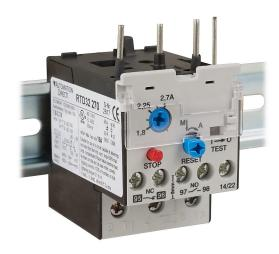
AutomationDirect RTD32 series thermal overload relay, 1.8-2.7A adjustable, bi-metallic, direct mount power connection(s), DIN rail mount. For use with GH15BN to GH15FT 45mm contactors.
