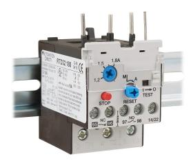
AutomationDirect RTD32 series thermal overload relay, 1.2-1.8A adjustable, bi-metallic, direct mount power connection(s), DIN rail mount. For use with GH15BN to GH15FT 45mm contactors.
