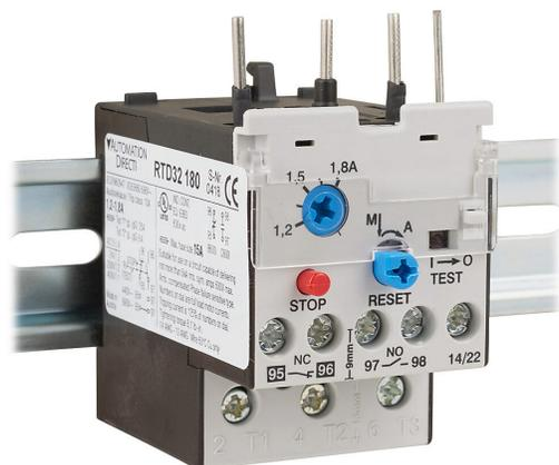
AutomationDirect RTD32 series thermal overload relay, 1.2-1.8A adjustable, bi-metallic, direct mount power connection(s), DIN rail mount. For use with GH15BN to GH15FT 45mm contactors.
