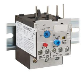
AutomationDirect RTD32 series thermal overload relay, 13.0-18.0A adjustable, bi-metallic, direct mount power connection(s), DIN rail mount. For use with GH15DN, GH15ET, or GH15FT 45mm contactors.
