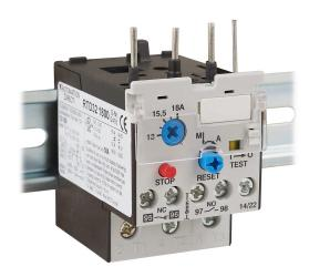
AutomationDirect RTD32 series thermal overload relay, 13.0-18.0A adjustable, bi-metallic, direct mount power connection(s), DIN rail mount. For use with GH15DN, GH15ET, or GH15FT 45mm contactors.
