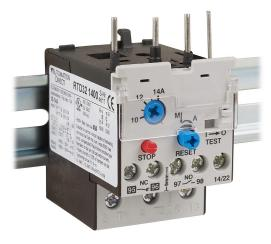
AutomationDirect RTD32 series thermal overload relay, 10.0-14.0A adjustable, bi-metallic, direct mount power connection(s), DIN rail mount. For use with GH15CN to GH15FT 45mm contactors.
