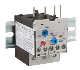
AutomationDirect RTD32 series thermal overload relay, 0.8-1.2A adjustable, bi-metallic, direct mount power connection(s), DIN rail mount. For use with GH15BN to GH15FT 45mm contactors.
