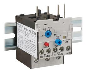
AutomationDirect RTD32 series thermal overload relay, 8.0-11.0A adjustable, bi-metallic, direct mount power connection(s), DIN rail mount. For use with GH15BN or GH15CN 45mm contactors.
