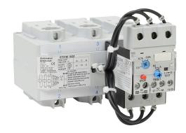
AutomationDirect RTD180 series thermal overload relay, 60.0-90.0A adjustable, bi-metallic, pass through connection(s), panel mount. For use with GH15KT, GH15LT or GH15MT 79mm contactors.
