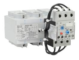
AutomationDirect RTD180 series thermal overload relay, 120.0-180.0A adjustable, bi-metallic, pass through connection(s), panel mount. For use with GH15NT or GH15PT 110mm contactors.
