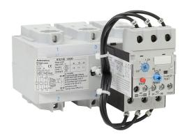
AutomationDirect RTD180 series thermal overload relay, 80.0-120.0A adjustable, bi-metallic, pass through connection(s), panel mount. For use with GH15LT or GH15MT 79mm contactors.
