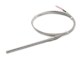
ProSense temperature sensor, Pt100 RTD, lead wire transition probe, 18in insertion length, 1/4in probe diameter, stainless steel sheath, 6ft 24 AWG wire leads.
