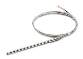
ProSense temperature sensor, Pt100 RTD, lead wire transition probe, 12in insertion length, 1/4in probe diameter, stainless steel sheath, 6ft 24 AWG wire leads.
