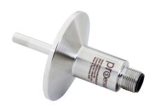
ProSense temperature sensor, Pt100 RTD, sanitary connection probe, 30mm insertion length, 6mm probe diameter, stainless steel sheath, 1-1/2in sanitary tri-clamp process connection, 4-pin M12 quick-disconnect.
