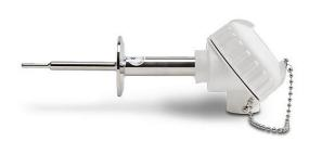
ProSense temperature sensor, Pt100 RTD, sanitary connection probe, 4in insertion length, 3/8in reduced to 3/16in probe diameter, stainless steel sheath, 2in sanitary tri-clamp process connection, white polypropylene screw cover head with terminals.
