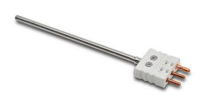
ProSense temperature sensor, Pt100 RTD, attached plug probe, 6in insertion length, 1/4in probe diameter, stainless steel sheath, 3-pin standard size plug.
