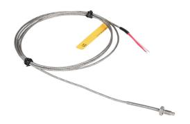
ProSense temperature sensor, Pt100 RTD, threaded bolt sensor, 3/8in bolt length, 3/16in tip, stainless steel sheath, 1/4-28 UNF process connection, 6ft 24 AWG wire leads.
