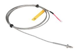
ProSense temperature sensor, Pt100 RTD, threaded bolt sensor, 3/8in bolt length, 3/16in tip, stainless steel sheath, 1/4-28 UNF process connection, 6ft 24 AWG wire leads.
